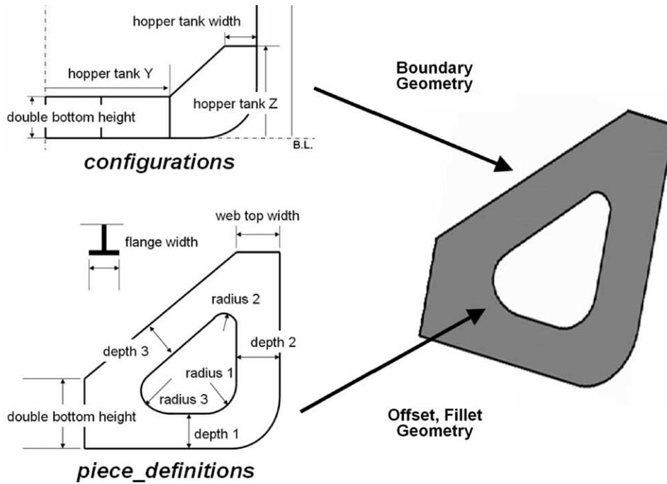
Fig. 10. Enhancement of hopper tank web plates.
