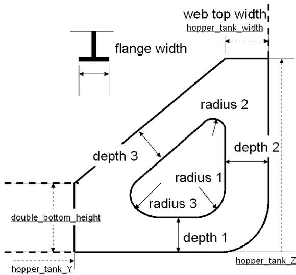
Fig. 5. Entity *piece\_definitions* of hopper tank web (transverse members).
