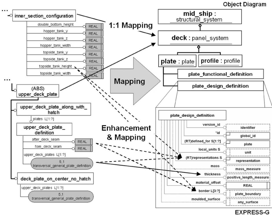
Fig. 8. Mapping the information model of midship drawing into STEP AP218.
