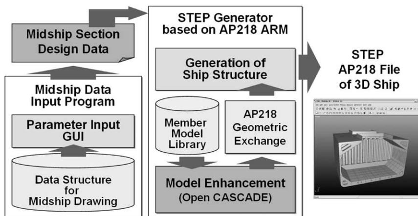
Fig. 1. Architecture of the 3D ship structure generation system.
