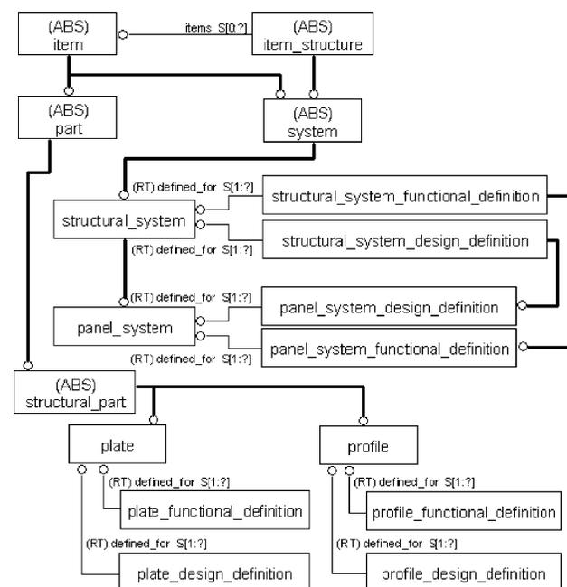
Fig. 2. Partial representation of AP218 structure.
