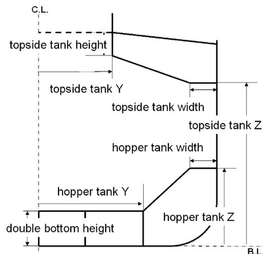
Fig. 4. Entity configurations of the inner section.
