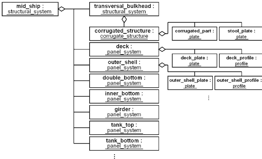
Fig. 11. UML object diagram of midship structure.
